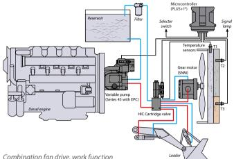
Combination fan drive, work function circuit using Series 45, PLUS+1®, and other Danfoss components
