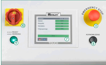
Operating elements of the tube forming machine
