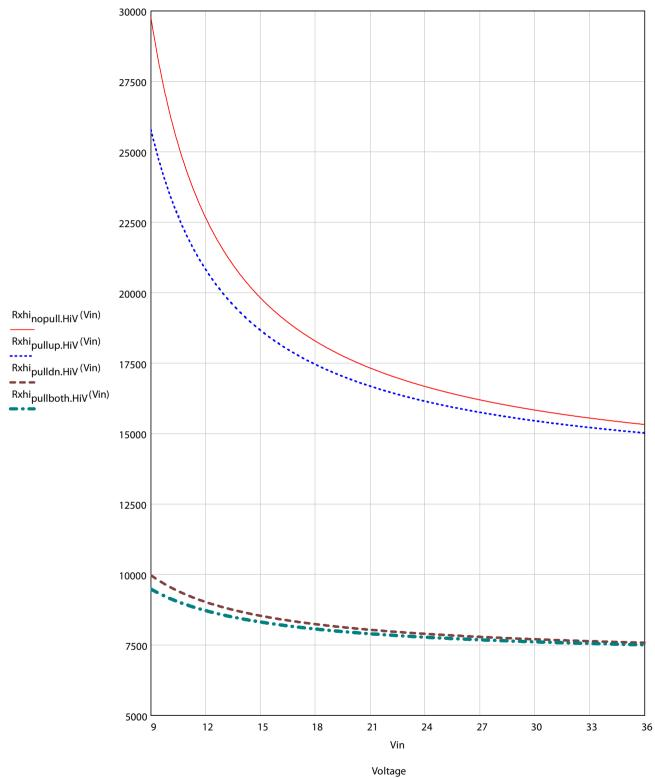
High range input impedance for analog inputs
