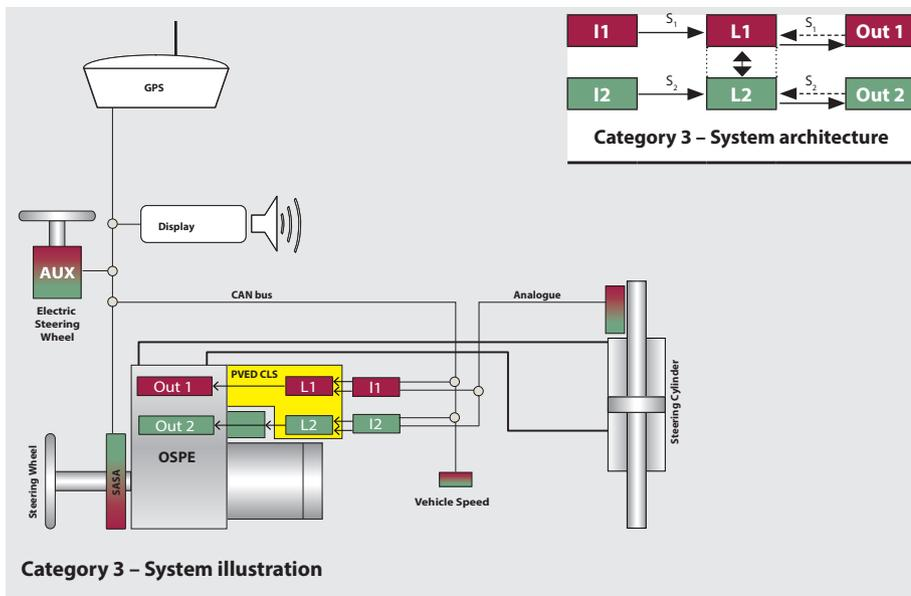
4 The safety function architecture is the minimum architecture required to meet the result of the hazard and risk analysis.
