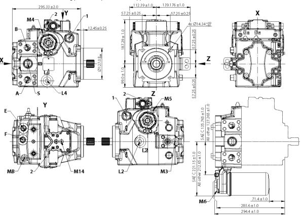
**A/B** system ports: Ø25.4 mm; M12 x 1.75; 20 min. full thread depth **MA/MB** (system), **M3, M6** (charge) gauge ports per ISO 11926-1:  $\frac{9}{16}$ –18 **M4, M5** (servo), **M14** (case) gauge ports per ISO 11926-1:  $\frac{7}{16}$ –20 **L2, L4** – Case drain ports per ISO 11926-1:  $1\frac{1}{16}$ –12
