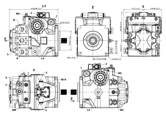
A/B system ports: Ø38 mm, 450 bar split flange boss per ISO 6162, M16 x 2; 27 min. full thread depth
