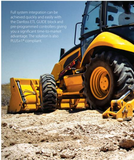
The Danfoss ETL control can be fitted into any existing pressure compensated/load sensing or mechanical torque control (MTC) system. Unlike other PCLS or MTC systems, the Danfoss solution is not limited by traditional sizing or engine torque constraints, but can operate in a full range of pump displacement and engine torque curves.
