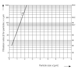
> 2  $\mu$ m Composite 99.5% efficiency for particles of size 2  $\mu$ m tested in a single pass test with ISO MTD
