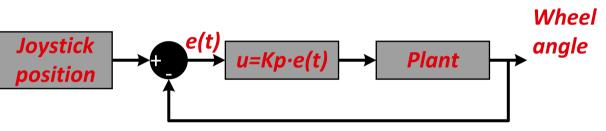
The joystick position corresponds to a wheel angle set-point. The closed loop controller works to minimize the error, thereby the wheel angle will follow the joystick position.
