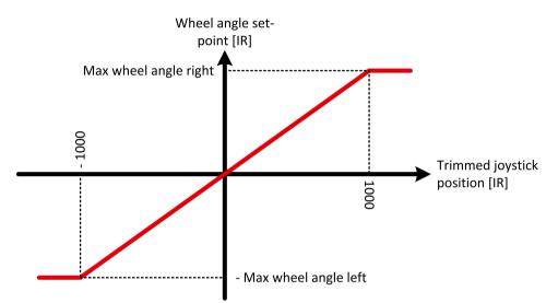
The wheel angle set-point and the measured wheel angle will be used to calculate the closed loop error.
