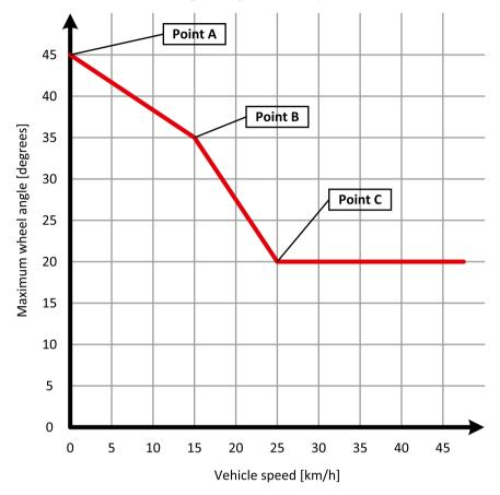
The following parameters are used to configure the piecewise linear function shown above:
