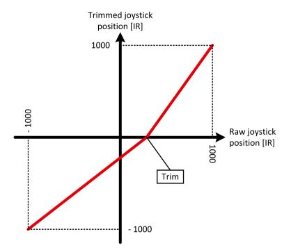
The example above shows a situation where the joystick neutral position has been trimmed to the right.
