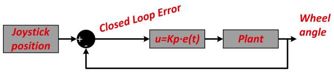
The output of the control loop is a flow set-point. Since a P-controller is used, the controller is represented by the following equation:
