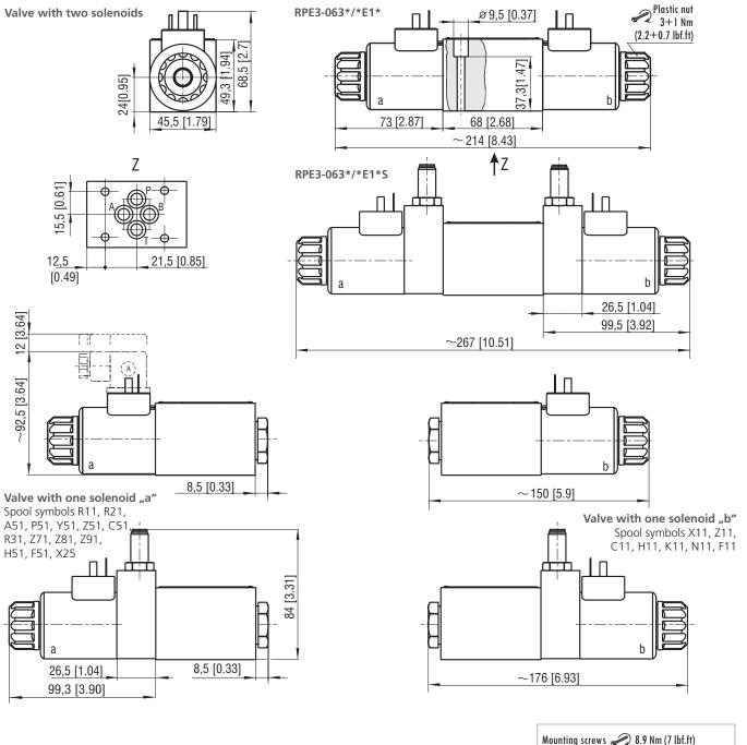
Mounting screws 28.9 Nm (7 lbf.ft) M5x45 DIN 912-10.9
